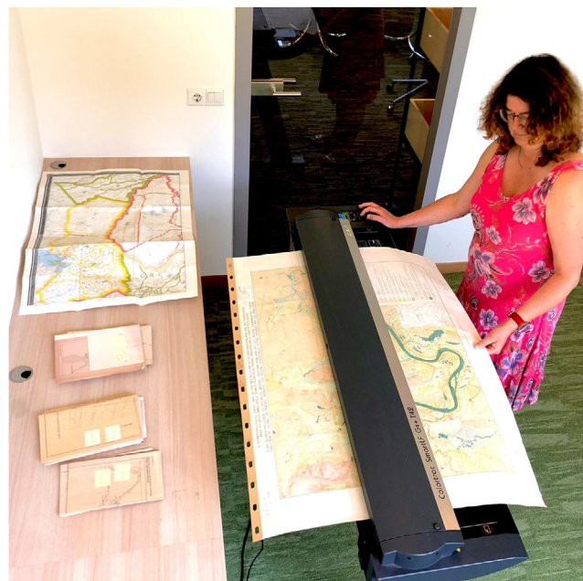
FIGURE 1 Digitization of a legacy soil map at International Soil Reference and Information Centre (ISRIC)—World Soil Information in the Netherlands in 2021. The operator places the soil map in a high-resolution scanner. A digital copy of the map is then rendered in the computer and manually georeferenced. The map is stored in a raster graphic format, which enable computer processing and manipulation in a geographic information system (e.g., to recreate mapping units). Picture courtesy of ISRIC—World Soil Information
