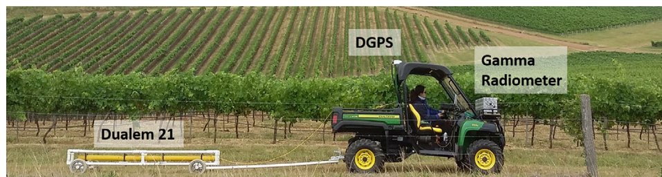
FIGURE 3 A multisensor soil sensing platform composed of a RSX-1 gamma spectrometer (Radiation Solutions) and an electromagnetic induction instrument (Dualem21; Dualem). The sensors are mounted on a field vehicle equipped with a high-precision differential GPS (DGPS) to sense the soil of a vineyard of the Pokolbin region in the lower Hunter Valley of New South Wales, Australia
